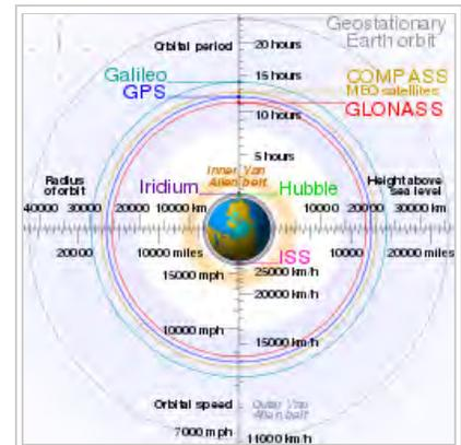
Comparison of geostationary, **GPS, GLONASS, Galileo, Compass (MEO)**, International Space Station, Hubble Space Telescope and Iridium constellation orbits, with the Van Allen radiation belts and the Earth to scale.<sup>[a]</sup> The Moon's orbit is around 9 times larger than geostationary orbit.<sup>[b]</sup> (In the SVG file, <http://upload.wikimedia.org/wiki/...> hover over an orbit or its label to highlight it; click to load its article.)
