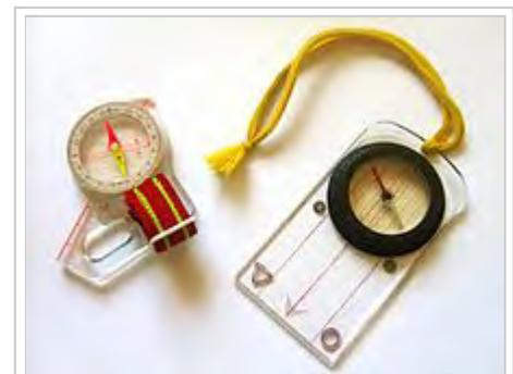
Thumb compass and protractor compass
