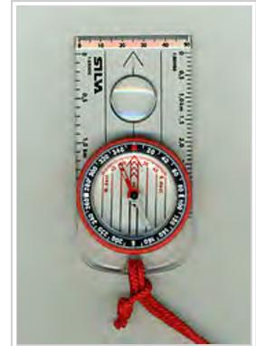
A liquid-filled protractor or orienteering compass with lanyard
