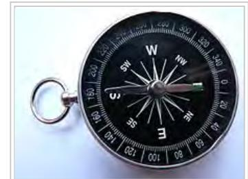
A simple dry magnetic portable compass
