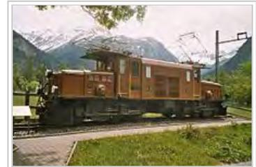
Swiss Rhaetian Railway Ge 6/6 I Krokodil locomotive, with a single large traction motor above each bogie, with drive by coupling rods.
