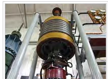
Rotor of a large water pump. The slip rings can be seen below the rotor drum.
