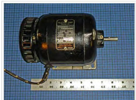
Single-phase 60 Hz 1800 RPM synchronous motor for Teletype machine, non-excited rotor type, manufactured from 1930 to 1955.
