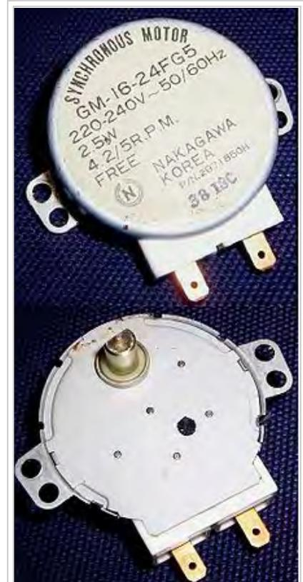
Small synchronous motor and integral stepdown gear from a microwave oven
