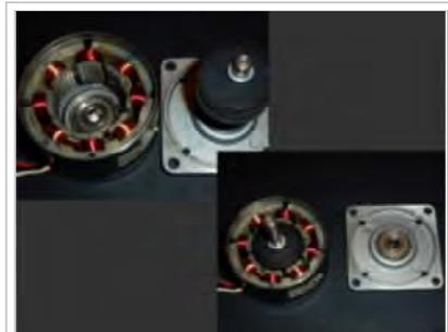
A bipolar hybrid stepper motor
