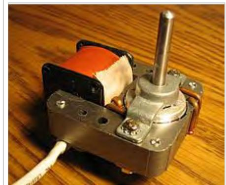
Small C-frame shaded-pole squirrel-cage motor. With the poles shown, the rotor will rotate in the clockwise direction.
