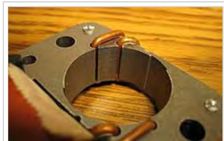
Shading coils (*copper bars*)
