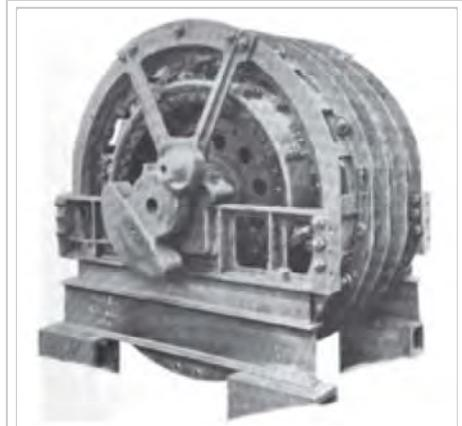
700 horsepower Brown-Boveri-Déri repulsion motor with 10 poles to be used with 16 2/3 Hz single phase current. Two of these motors were used in the French electric locomotive Midi E3301
