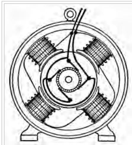
Consequent field, four-pole, shunt-wound DC generator
