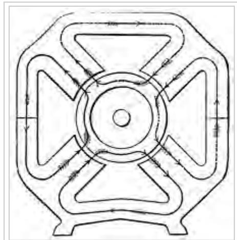
Field lines of a four-pole stator passing through a Gramme ring or drum rotor.
