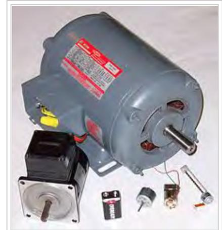
Various electric motors, compared to 9 V battery.
