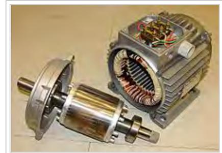
Electric motor rotor (left) and stator (right)
