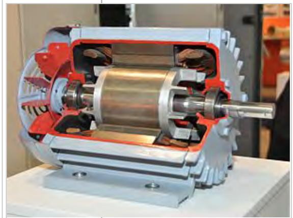
Cutaway view through stator of induction motor.
