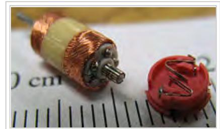
A toy's small DC motor with its commutator
