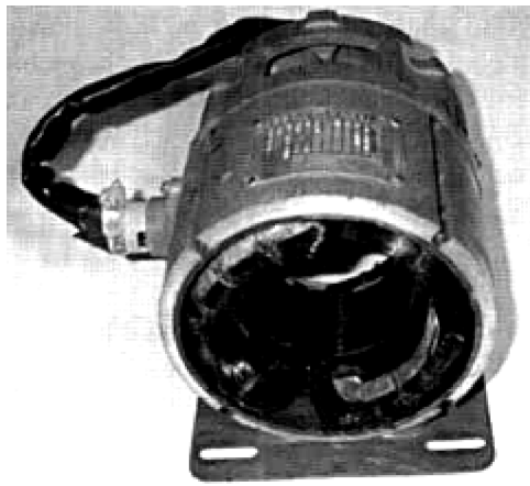
FIGURE 12-3 The stationary part of a DC motor has the field coils mounted in it.
