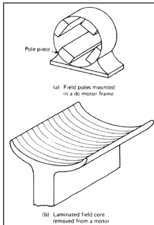
**FIGURE 12-8 (a) This diagram shows the location of the pole pieces in the frame of a DC motor. (b) This diagram shows an individual pole piece. You can see that it is made of laminated sections. The field coils are wound around the pole pieces.**
