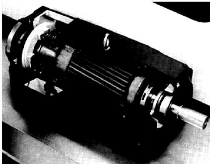
FIGURE 12-5 A cutaway picture of a DC motor.
