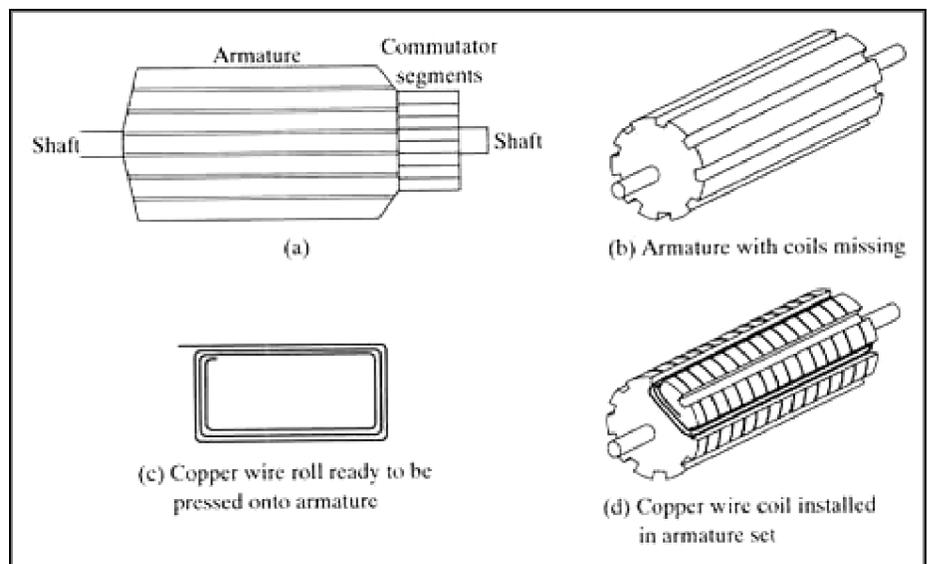
**FIGURE 12-7 (a) Armature and commutator segments. (b) Armature prior to the coil's wire being installed. (c) Coil of wire prior to being pressed into the armature. (d) A coil pressed into the armature. The end of each coil is attached to a commutator segment.**
