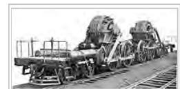
The Pennsylvania Railroad's class DD1 locomotive running gear was a semi-permanently coupled pair of third rail direct current electric locomotive motors built for the railroad's initial New York-area electrification when steam locomotives were banned in the city (locomotive cab removed here).
