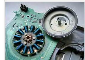
The motor from a 3.5" floppy disk drive. The coils, arranged radially, are made from copper wire coated with blue insulation. The rotor (upper right) has been removed and turned upside-down. The grey ring inside its cup is a permanent magnet.
