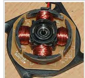
The four poles on the stator of a two-phase brushless motor. This is part of a computer cooling fan; the rotor has been removed.
