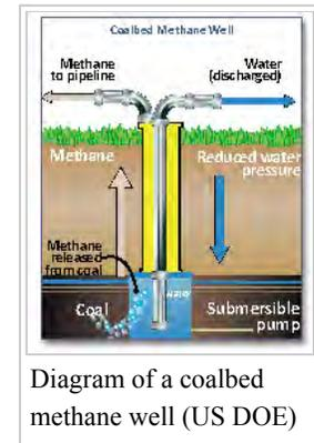
Diagram of a coalbed methane well (US DOE)
