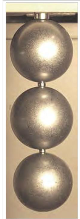
Neodymium magnets (small cylinders) lifting steel balls. As shown here, rare-earth magnets can easily lift thousands of times their own weight.
