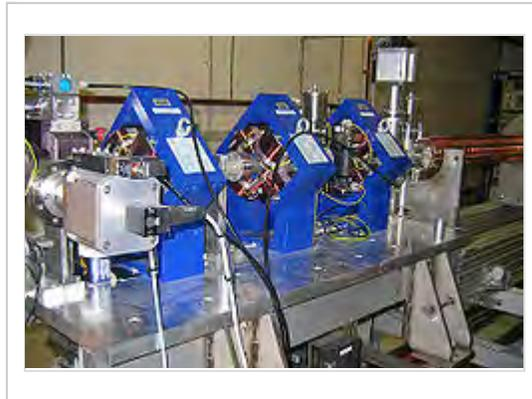
Quadrupole electromagnets (in blue), surrounding the linac of the Australian Synchrotron, are used to focus the electron beam
