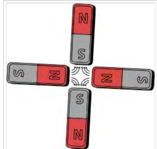
Four bar magnets configured to produce a quadrupole
