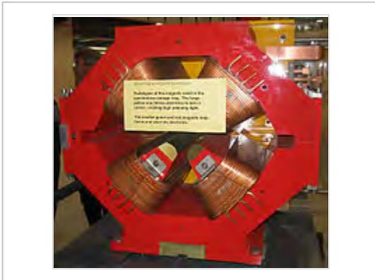
A quadrupole electromagnet as used in the storage ring of the Australian Synchrotron
