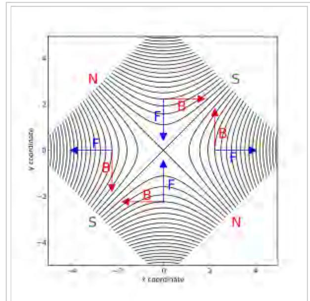
Magnetic field lines of an idealized quadrupole field in the plane transverse to the nominal beam direction. The red arrows show the direction of the magnetic field while the blue arrows indicate the direction of the Lorentz force on a positive particle going into the image plane (away from the reader)
