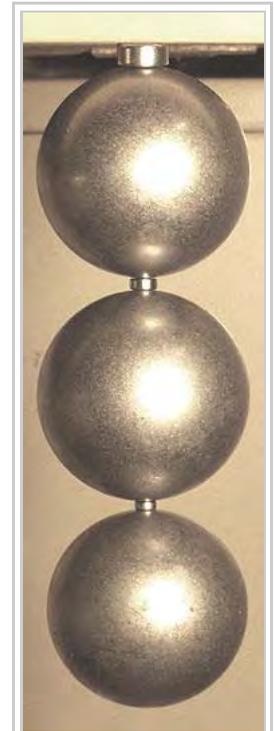
Neodymium magnets (small cylinders) lifting steel spheres. Such magnets can easily lift thousands of times their own weight.
