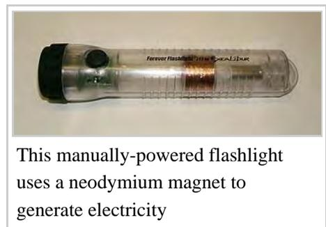
This manually-powered flashlight uses a neodymium magnet to generate electricity
