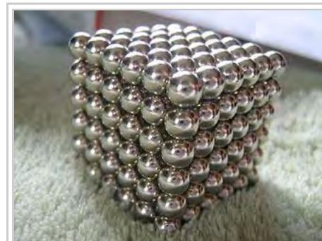
Neodymium magnet spheres assembled in the shape of a cube
