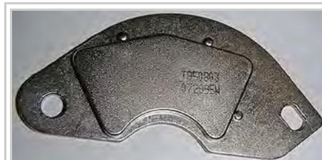
Nickel plated neodymium magnet on a bracket from a hard disk drive
