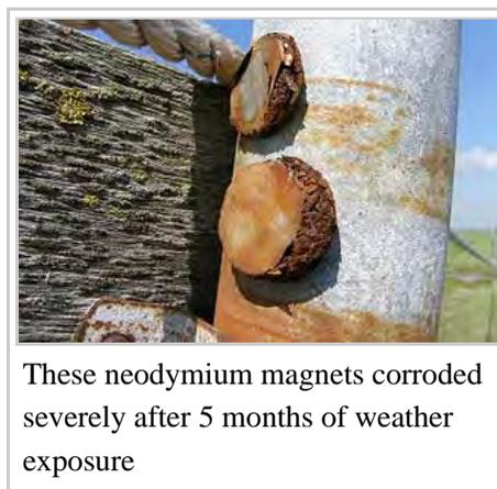
These neodymium magnets corroded severely after 5 months of weather exposure
