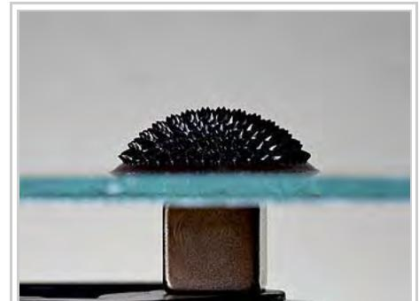
Ferrofluid can be used to disclose a powerful neodymium magnet's field
