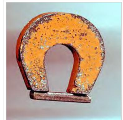
A "horseshoe magnet" made of alnico, an iron alloy. The magnet, made in the shape of a horseshoe, has the two magnetic poles close together. This shape creates a strong magnetic field between the poles, allowing the magnet to pick up a heavy piece of iron.
