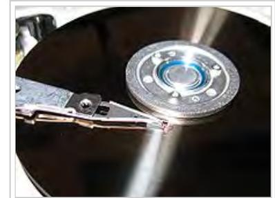
Hard disk drives record data on a thin magnetic coating
