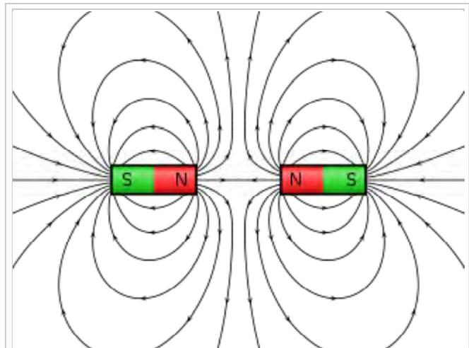
Field of two repelling cylindrical bar magnets
