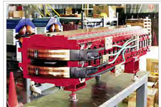
Dipole magnet from the Advanced Photon Source
