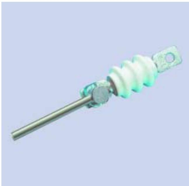
The spark gap consists of two electrodes arranged at a defined distance from each other in a ceramic housing. Type 482 satisfies the requirements of degree of protection IP 54.
