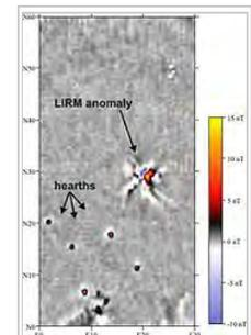
Lightning-induced remanent magnetization (LIRM) mapped during a magnetic field gradient survey of an archaeological site located in Wyoming, United States.
