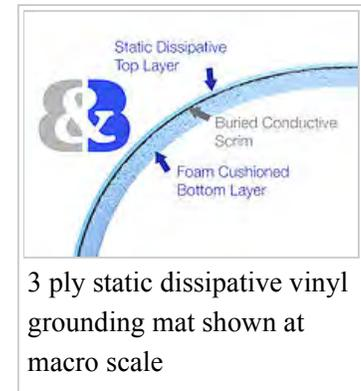
3 ply static dissipative vinyl grounding mat shown at macro scale
