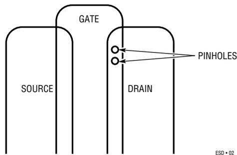
This failure mechanism can also be found on bipolar ICs which have metallization runs over active semiconductor regions separated by a thin oxide. Device failures are characterized by resistive or high leakage paths.
