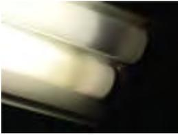
First and foremost... look at the bulbs! If either bulb appears to be very dark near either end the bulb is defective or close to failure. Note the upper bulb in the left graphic... it is definitely approaching its golden years! Though this bulb is still producing light its days
