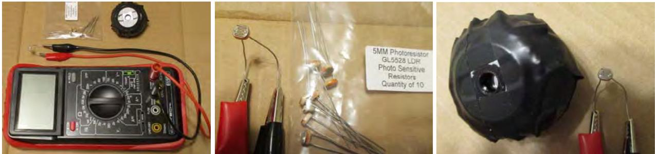
This UVC light sensor (shown on the right above) was made using (front to back) a fender washer with a ¼" hole in it, then the UV pass ban filter then the photo resistor. This was embedded in black foam rubber. Enough black tape was used on the outside to keep light from coming in form the side. Sun light being very high intensity parallel waves from one direction was used to test for leakage by slowing turning the sensor to different direction and watching the ohm meter.
