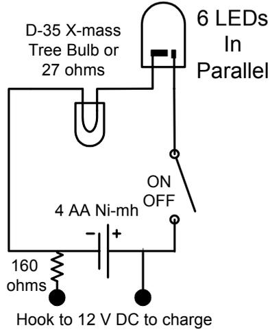
The clip was salvaged from a small clip-on LED “astro lite” bought at a 99 cent store. It was cut down to size with a hack saw. A pc board with holes in it was cut to size and 6 white LEDs were wired in parallel as per the diagram and picture above. 5 min epoxy was used to hold the LEDs in place. Silicon rubber gasket sealer was used to hold the resistor or x-mass tree bulb and charging leads in place.
