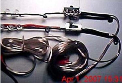
The use of a PC board with holes in it worked the best to organize and point the LEDs. Note that this rendition uses the LM-317 to limit current to 84 ma.
