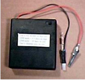
The clip is used to change from high to low setting. The switch on the battery case is used to turn on and off the unit. Other colors like amber are also useful to help keep bugs away at night.
