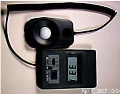
Another more accurate way to measure total light output energy is to use a silicon photo cell inside a small black box with a hole the size of the LED in one side. The arrangement is such that the LED is held close but at a fixed
