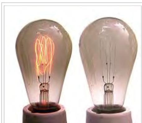
Carbon filament lamps, showing darkening of bulb
