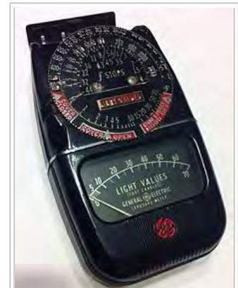
General Electric Light Meter used in photography to measure light values in foot candles.
