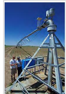
The hub of a center-pivot irrigation system
