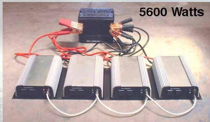
Each power inverter in the stackable modular array is rated at 1400 watts.
