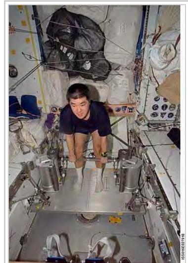
Exercise in space: Astronaut Daniel Tani, Expedition 16 flight engineer, works out at the Unity node of the International Space Station using the short bar of the Interim Resistive Exercise Device (IRED) to perform pull-ups to increase his upper body strength while in a microgravity environment
