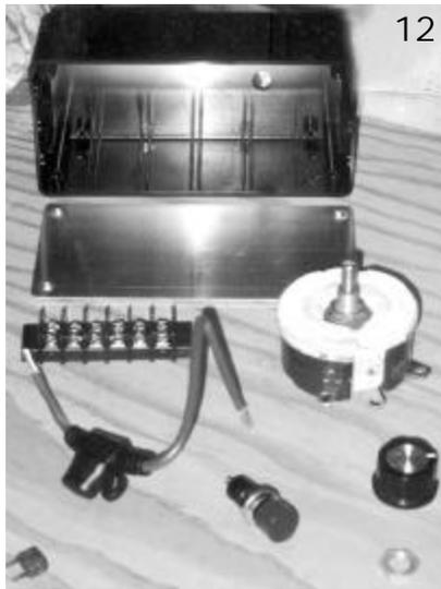
Fig. 12: Components for the control box are based on the circuit illustrated in Fig. 11.
