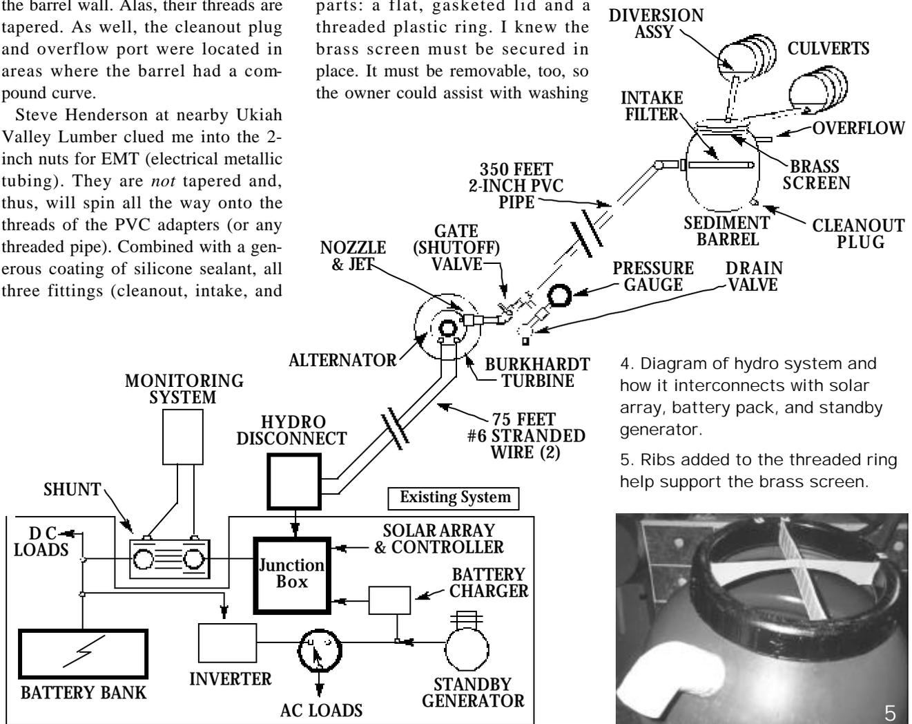
4. Diagram of hydro system and how it interconnects with solar array, battery pack, and standby generator.
