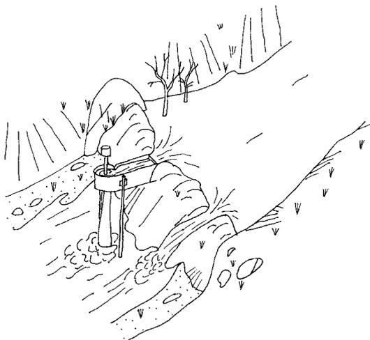
Dams have both advantages and disadvantages. If used in a village setting they can provide additional uses as a fish pond and washing area. The dam wall may support a row of PowerPal generators so that several families can have access to electricity. If the village works together to build the dam the time and construction costs are lower. Dams are less likely to be effected by flooding if diversion channels are adequate, so PowerPal can be used effectively during the rainy season.
