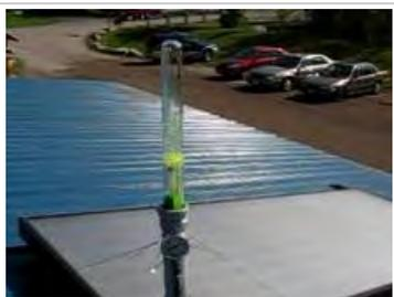
The bubble separator of a bubble-pump system
