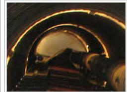
View of the silo unloader drop chute inserted into the very top of the silage drop tube 60ft up. The tube is illuminated by light entering through fiberglass panels every 20ft along the outer steel shroud.
