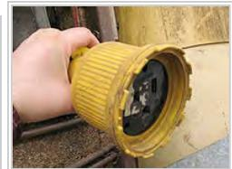
50 amp, 250 volt unloader power socket, with shroud to keep out debris.
