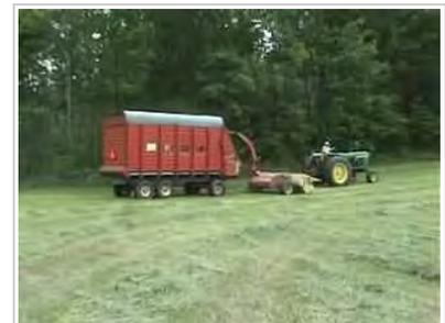
320x240 200kbit/s video of a PTO-driven towed New Holland forage harvester, John Deere 4020 tractor, and Gehl forage wagon. See also: High detail 600kbit/s 640x480
