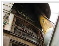
View of silo unloader doors, silage drop tube, and paddle conveyor leading into barn.
