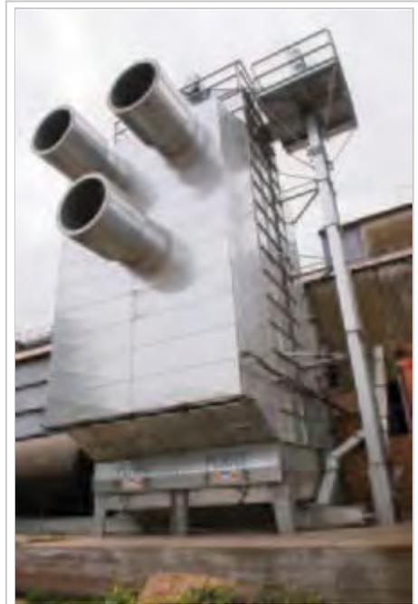
Continuous mixed flow grain dryer
