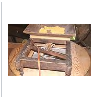
"Slipper" feeding corn into the grindstones of George Washington's Grist Mill
