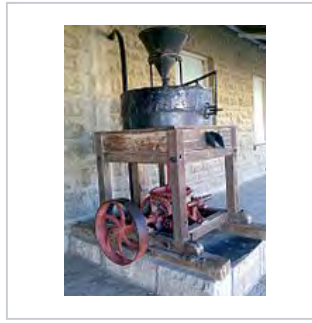
Grain mill with bevel gears outside local museum at Dordrecht
