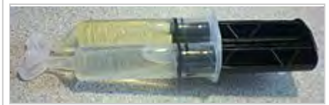
A syringe of "5-minute" epoxy glue, containing separate compartments for the epoxy resin and the hardener.
