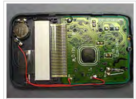
The interior of a pocket calculator. The dark lump of epoxy in the center covers the processor chip
