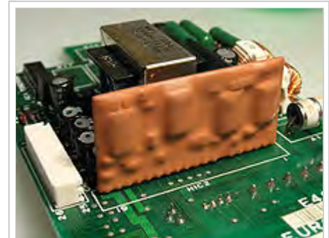
An epoxy encapsulated hybrid circuit on a printed circuit board.
