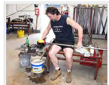
A stage in the manufacture of a Bristol blue glass ship's decanter. The blowpipe is being held in the glassblower's left hand. The glass is glowing yellow.
