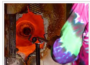
Use of a glory hole to reheat a piece on the end of a blowpipe
