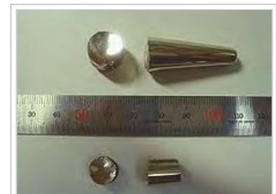
Samples of amorphous metal, with millimeter scale
