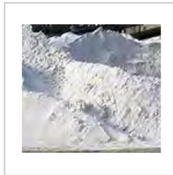
Quartz sand (silica) is the main raw material in commercial glass production
