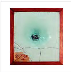
Mouth-blown window-glass in Sweden Kosta Glasbruk, (1742) with a pontil mark from the glassblower's pipe
