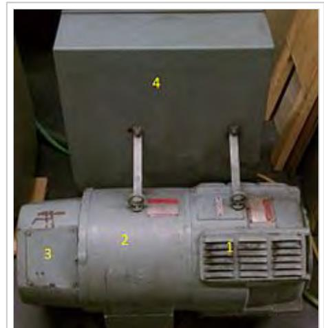
An MG set used to provide a variable three phase AC voltage for an Electron Beam Welding Machine high voltage power supply.
