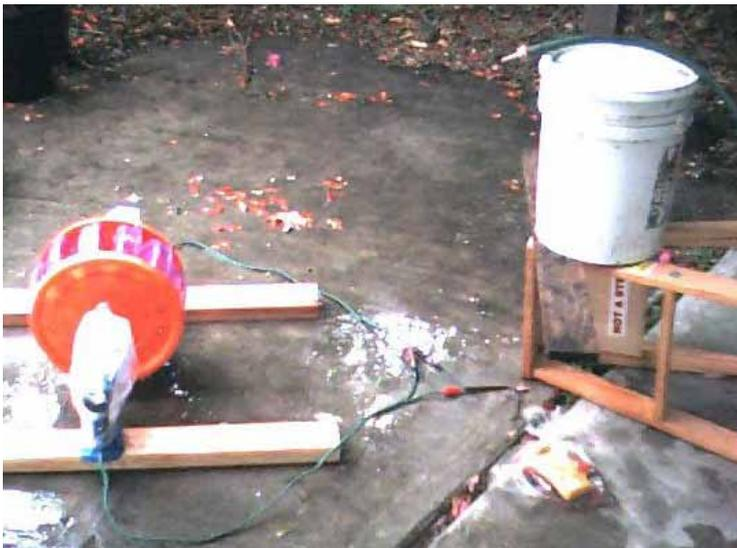
Next I tested output for two sets or 24 cups making two water wheel driving two 14.4 volt cordless drills. I measured between .5 to 2.9 amps (or .8 to 5.2 watts) charging one cell. Both generators were wired in series.
