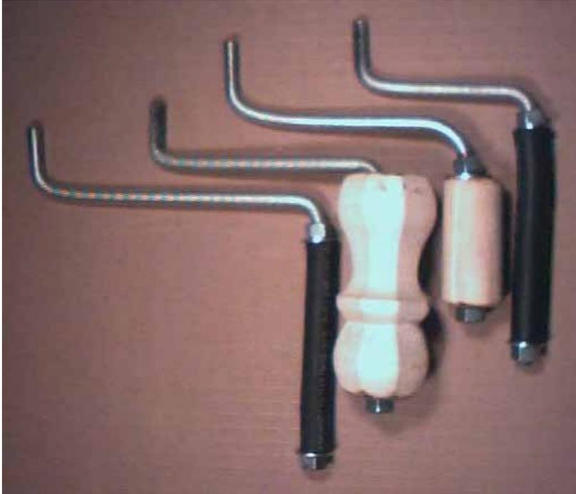
Drill weight is about 2.1 lbs with lead wire. Crank is about 8 Ozs.
