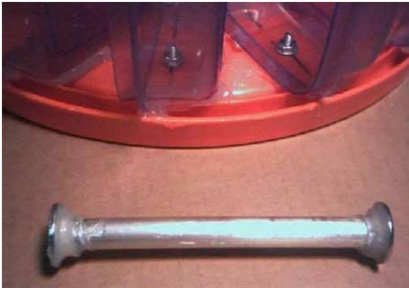
Use this pipe as a spacer between the lids in the center when assembling the last side. One water wheel weight is about 3 lbs two is about 5 lbs. Caution: the 3/8” shaft will bend if nuts are tighten against a pipe that has a non-square end. Use a pipe cutter and get a square end. Don’t use a hacksaw. See <http://home1.gte.net/mikelob/WaterW-6.JPG>
