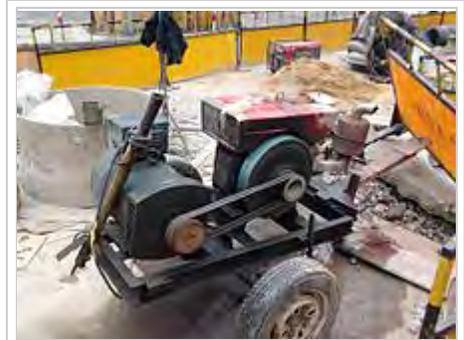
Cart-mounted engine-generator being used at a construction site
