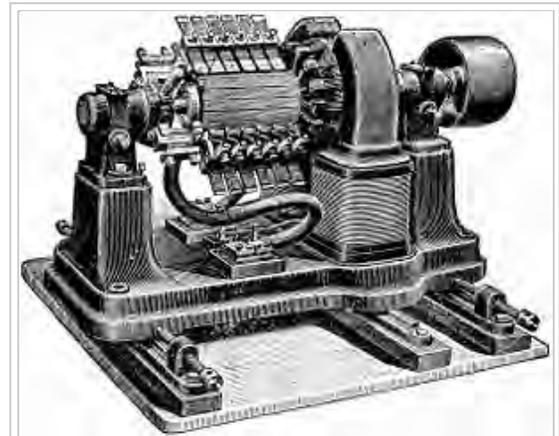
This large belt-driven high-current dynamo from around 1917 produced 310 amperes at 7 volts DC. The huge complicated commutator (*left*) was needed to handle the large current. Dynamos are no longer used due to the size and complexity of commutators needed for high power applications.
