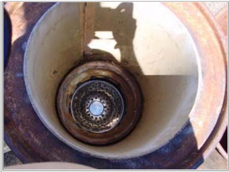
**a view down into the gassifier core**
