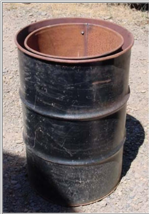
The design we're building is called a "down-draft generator," and construction-wise, it can be described as a tank within a tank within a tank.
