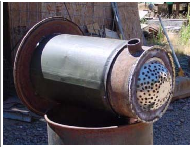
the gassifier core shown laying on its side with the reduction bowl and retaining ring installed
