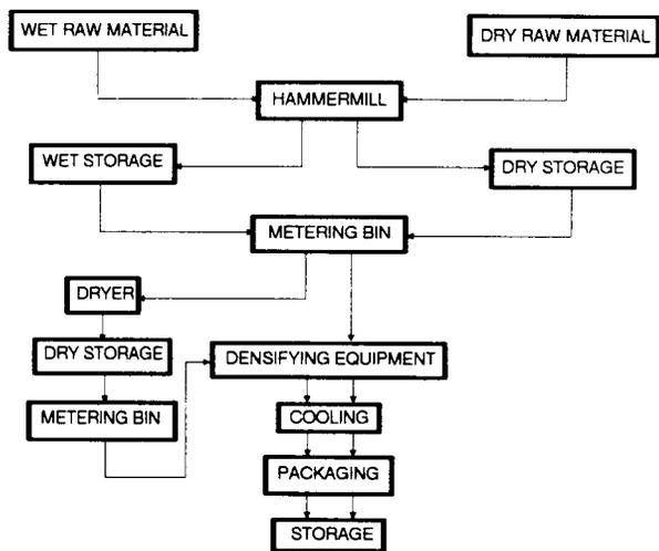
Fig. 3 Flow Diagram for Wet and Dry Materials
