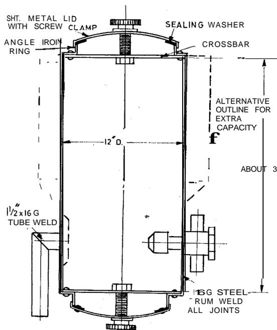
*Above, Fig. 4: Distemper drum producer; and right, Fig. 5: Final design of gas producer*
